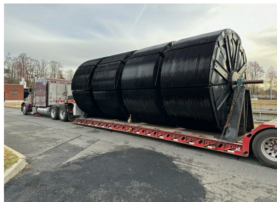
New Rotating Biological Contactors (RBC's) arriving at plant to replace broken units.
